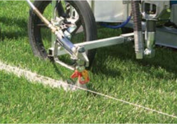
The FieldLazer S100 uses airless technology for spraying brighter, longer-lasting lines.
