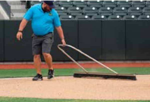
The super-wide Infield Drag Broom brings a leveling bar on one side and smoothing bristles on the other.
