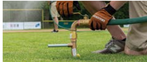
A Quick Coupler Key makes watering your field so much easier, and the ball valve eliminates back spray.
