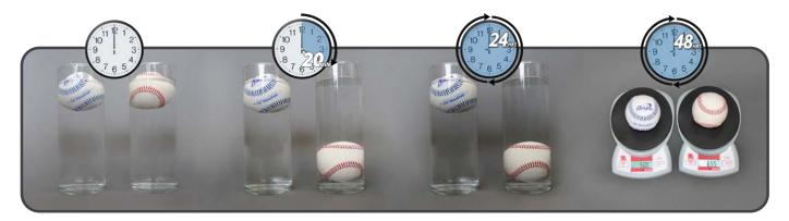
The All Weather ball and the traditional ball are placed into water at the same time. After 20 minutes the traditional ball sinks due to moisture absorption while the All Weather ball is still afloat.
