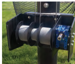
Winch and cable designed for single-person operation
