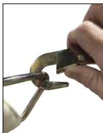
Attach net ring to Upright #2 cable with winch
