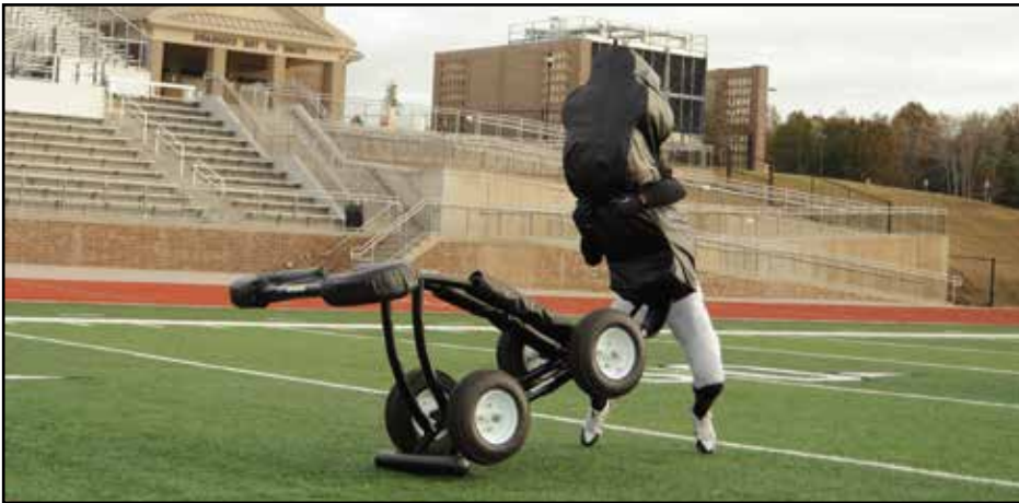
The player contacts the moving sled. When the front of the sled is raised 2" off the ground, the brake at the back of the sled engages the turf and stops the sled from rolling backwards.
