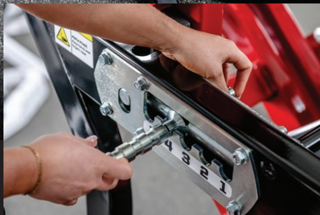
S.E.T. range limiter defines maximum depth
